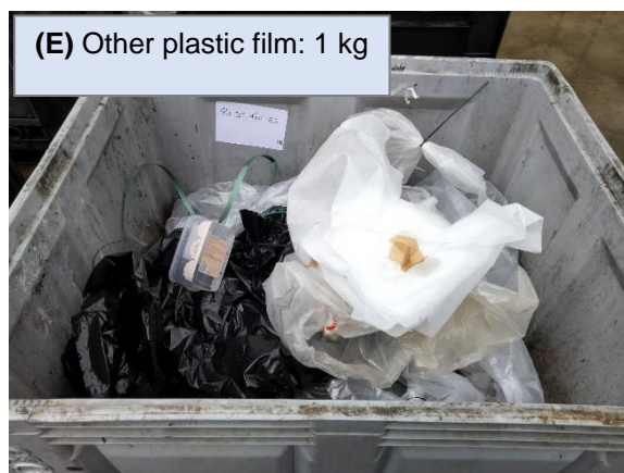
Figure 2. A few images of the collected samples from Construction sector (e.g., NACE sector F.41) from urban areas of Ghent, , consisting of Transparent PE Film (A), Colored PE Film (B), Transparent PP Film (C), Colored PP Film (D), and Other Plastic Film (E). More information on the samples is available in SI-section 4.
