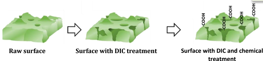
Biosorbents preparation by Instant Controlled Pressure Drop (DIC) and chemical treatment.
